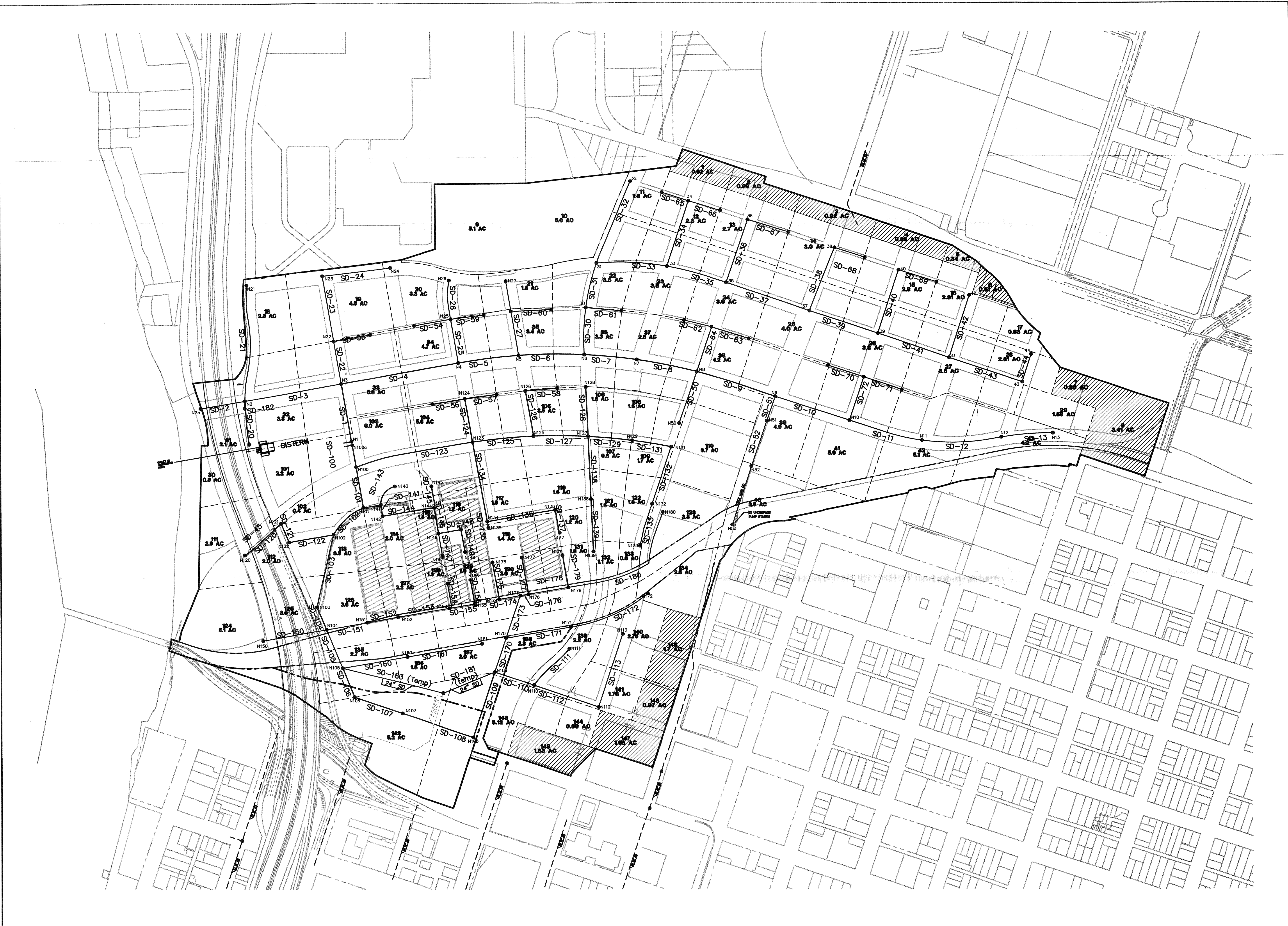
FIGURE 6 DRAINAGE SUBSHEDS, NODES & PIPE SEGMENT NUMBERS
