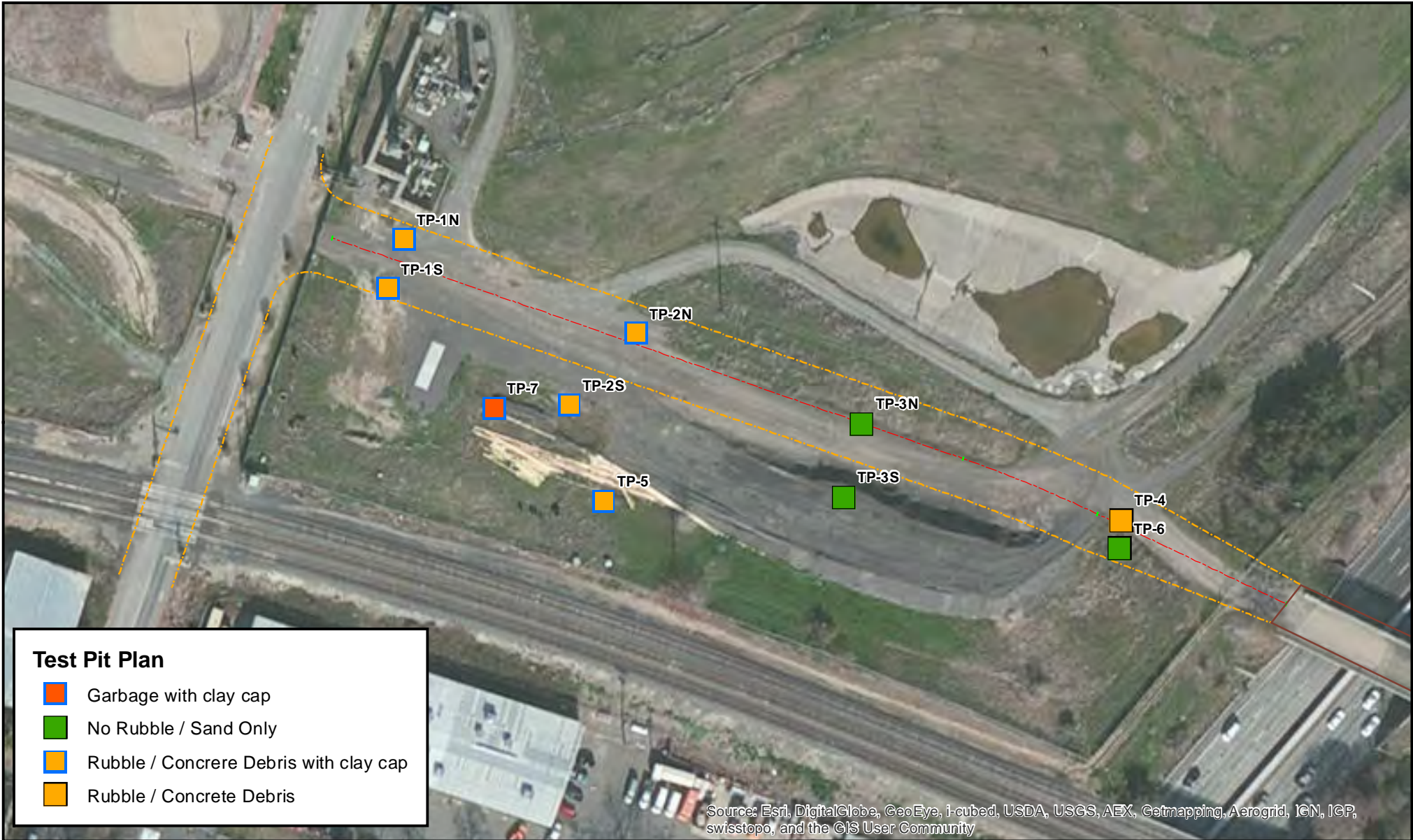
PLATE A-1 AERIAL VIEW AND APPROXIMATE TEST PIT LOCATIONS MCKINLEY VILLAGE A STREET IMPROVEMENTS SACRAMENTO, CA JANUARY, 2014 NOTES
