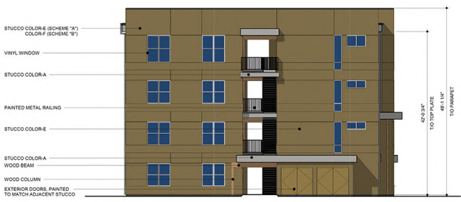
3 LEFT ELEVATION - BUILDING 1 3/32" = 1'-0"
