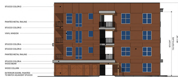
4 RIGHT ELEVATION - BLDG 2 3/32" = 1'-0"
