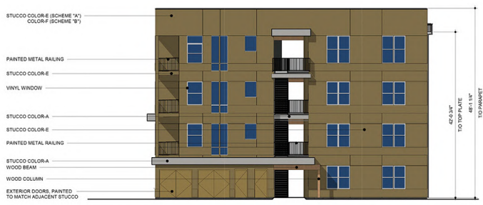
4 RIGHT ELEVATION - BUILDING 1 3/32" = 1'-0"
