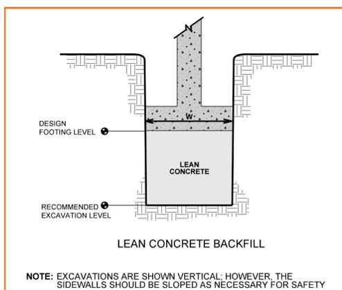
To ensure foundations have adequate support, special care should be taken when footings are located adjacent to trenches. The bottom of such footings should be at least 1 foot below an
