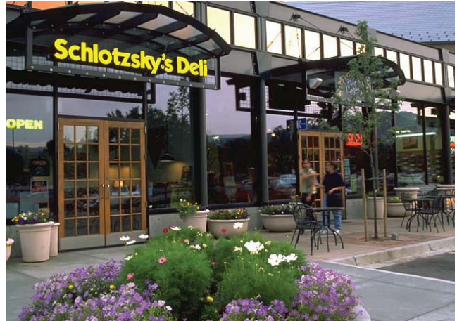
Color of letter returns should contrast with face colors for optimum daytime readability.
