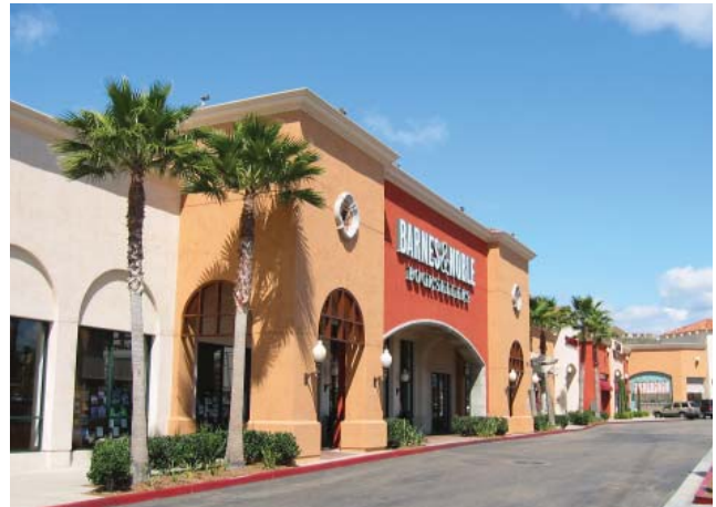
Building base should be visually anchored by use of articulated materials, architectural details or colors at the pedestrian level.
