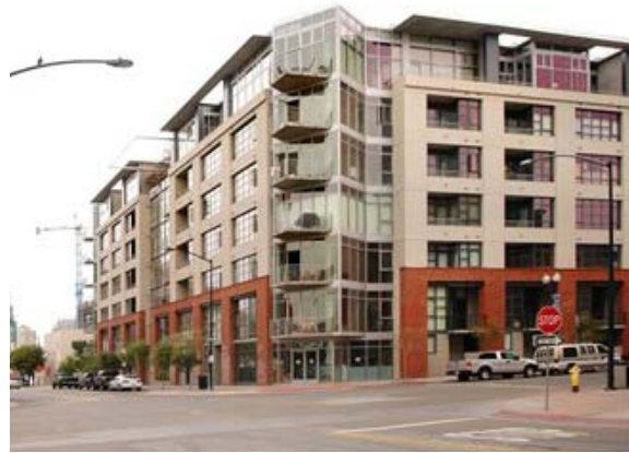
Façade treatment along the street should articulate the base, middle, and roof line.
