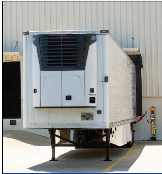
Figure 5: Photograph of Trailer-Mounted Electric Transport Refrigeration Unit (eTRU)
