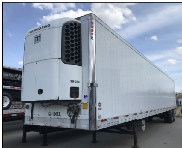
Figure 4: Photograph of a Trailer-Mounted Transport Refrigeration Unit (TRU)
