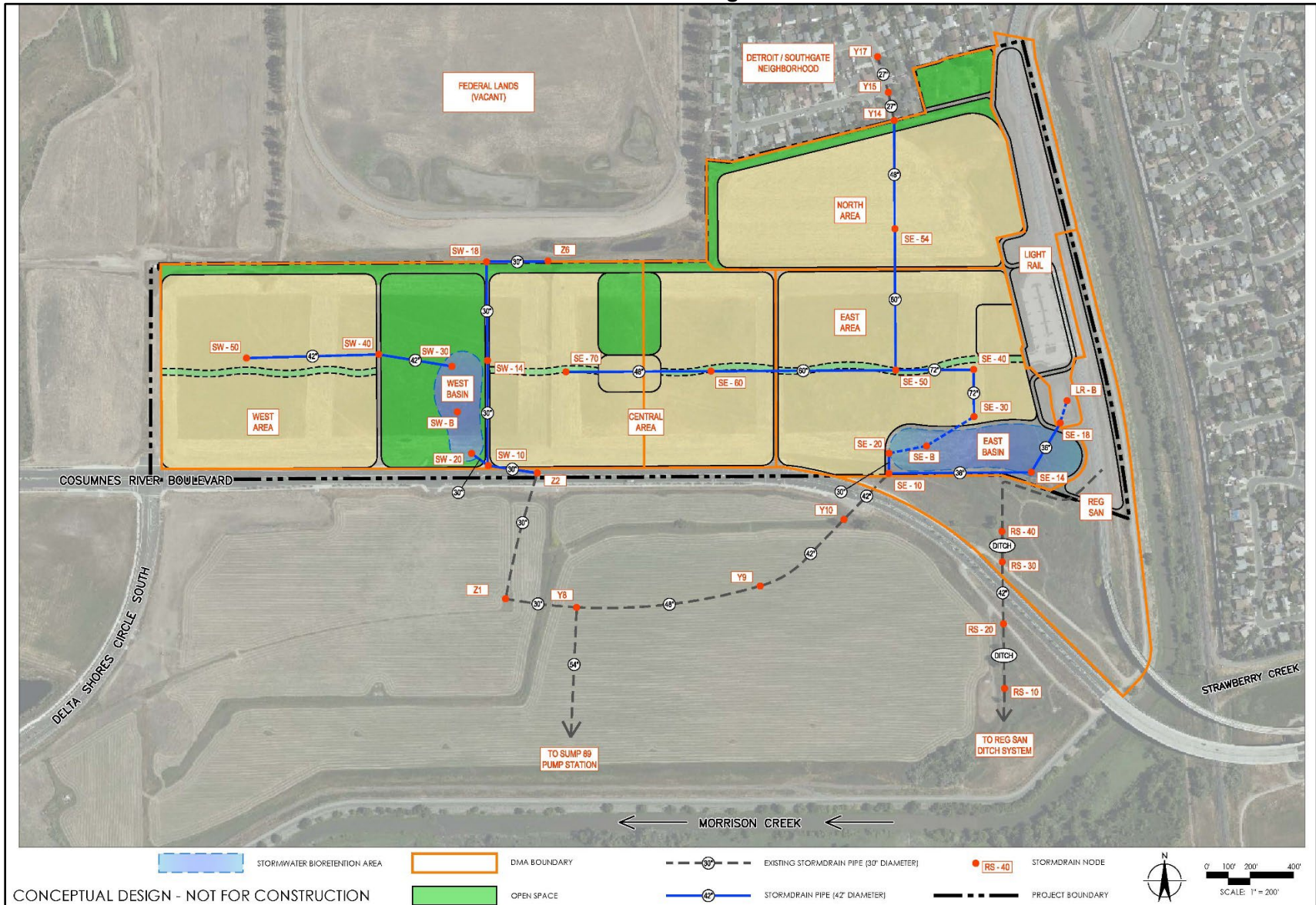
Figure 19 Stormwater Drainage Plan
